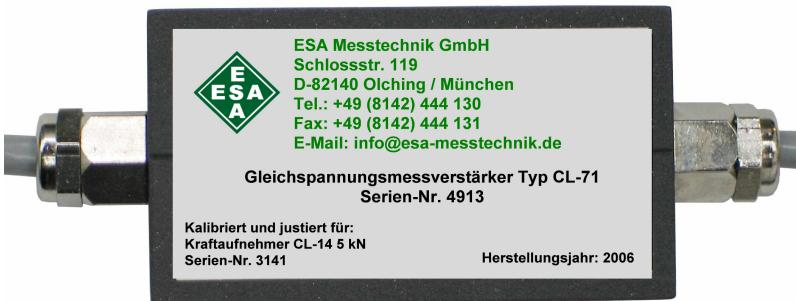
Mod. CL 71 is an ideal amplifier unit for strain gauge based pressure sensors, load cells and force sensors in unipolar measuring mode, i.e. either in tension or in compression. Its input circuitry is compatible with 120 Ω to 1200 Ω strain gauge full bridge configurations.
